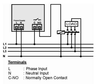
Figure -1 Connection Diagram
